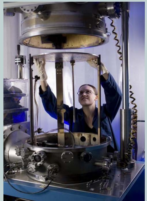
BYU Student Amy Baker was part of a team of undergraduates who built a specially coated mirror that will be launched into space onboard the Venus Express. Baker is shown here with the device used to apply the mirror's coating of chromium and magnesium fluoride.
