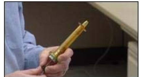
A syringe-like device is easily used in one hand, even by a first responder wearing gloves and protective clothing. He pushes the plunger, and a small metal fiber coated with a polymer film comes out to soak up whatever's out there.
